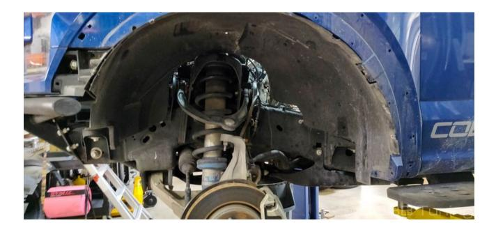
4. Using your fingers or a pick, remove the wiring for the side marker and set the fender flare somewhere safe.
