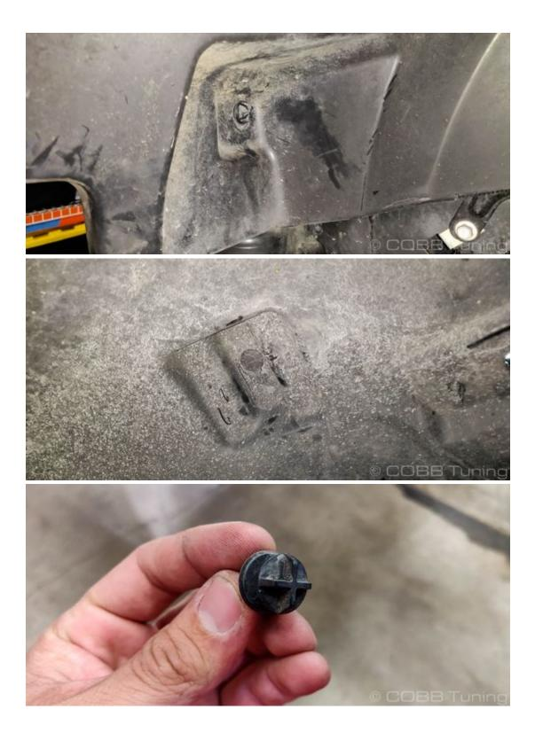
7. The liner can come out at this point and be set aside. You'll need to twist it a little bit in order to remove it from the weird bump on the front holding it in place.
