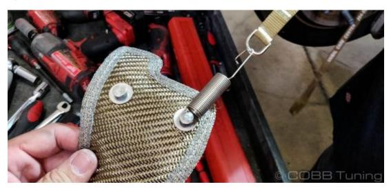
2. Using the provided wire or a random dog leash like we had lying around, fish through the turbo around the back side looping it around the spring before pulling it through slowly.
