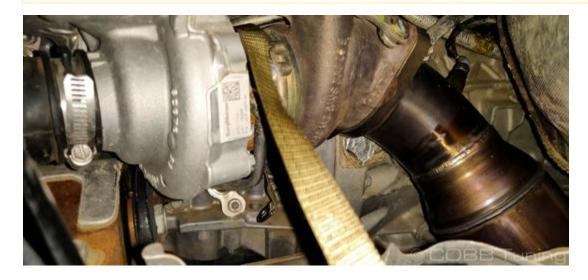
3. Slip the front side under the wastegate arm and attach the spring over the top. As well as the one attached to your pulling device to the one on the other side of the center housing.
