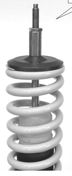
Assemble the factory bearing rubber and the center disc, as shown on the picture and mount the coilover strut with the factory parts to the chassis like the original suspension. Tightening torque 25Nm (18 ft-lb). Install the strut in the vehicle as specified by the vehicle manufacturer in their document.
