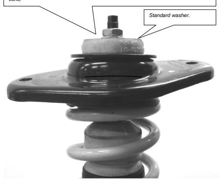
The original HA supporting bearing has a mark for the righte side = R and the left side = L. Please installation the Supporting bearing on the corect side.
