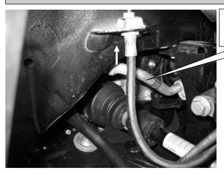
For enough distance between the driveshaft and the air conditioning pipe bend the air conditioning pipe 20 mm upwards. If it possibly to dismantle the holder of the air conditioning pipe.
