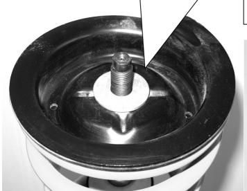
Install the factory supporting bearing and fix it with the supplied stop nut. Tightening torque for the piston rod nut is 50 Nm (37 ft-lb). The strut unit has to be installed according to manufacturers recommended settings regarding tightening torque and fixing specifications.
