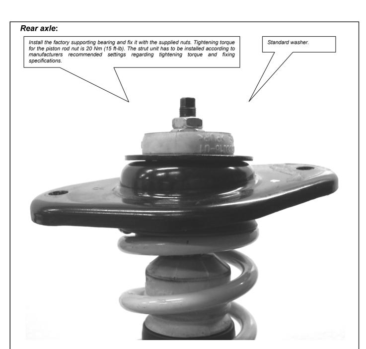
The original HA supporting bearing has a mark for the righte side = R and the left side = L. Please installation the Supporting bearing on the corect side.
