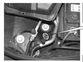
Please pay attention while dismantling the front axle strut! Remove the locking plug (black rubber part) in the engine area next to the battery. Dismantle the now visible screw/nut at the axle. DO NOT DISMANTLE the suspension arm as otherwise extensive measurement work has to be done on the front axle!
