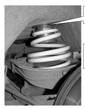
The height adjustment has to be inserted at the top and the original upper spring support has to be removed. Re-use the original rubber unit at the bottom end of the spring. Please read the height adjustment for adjusting the car height.
