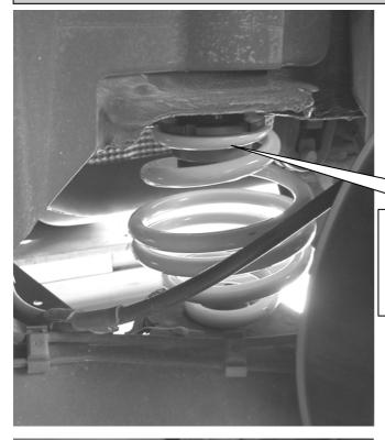
Insert the rear axle height adjustment at the top side of the chassis. The height adjustment perch has to be dismantled for changing the car height on the rear axle. The original spring base has to be removed.
