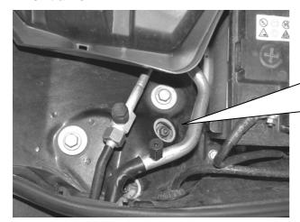
Please pay attention while dismantling the front axle strut! Remove the locking plug (black rubber part) in the engine area next to the battery. Dismantle the now visible screw/nut at the axle. (Maybe the locking plug has to be replaced by a new one: VW part no. N 102 265 01) DO NOT DISMANTLE the suspension arm as otherwise extensive measurement work has to be done on the front axle!
