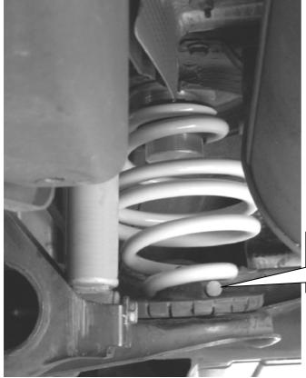
The spring has to be positioned so that the lower end of the spring shows to the right side of the car. The standard spring base has to stay installed.
