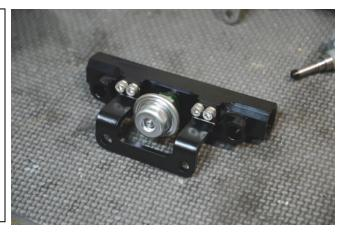
12. For 20-0111-00 or 20-0111-PK, install the included -6AN adapters into each end of the fuel rail, as shown. **To prevent failure, all O-rings MUST be lubricated prior to assembly.** Hold the fuel rail in a vice with non-marring jaws, and tighten the fittings with a 1" non-marring wrench.
