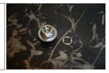
10. For 20-0111-PK or 20-0111-00 is used, install the fuel pulse damper adapter into the center port of the Radium fuel rail. Make sure the side that screws into the rail has an O-ring on it. To prevent failure, the O-ring MUST be lubricated prior to assembly.
