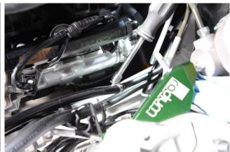
18. Connect the other end of the hose to the LH fuel rail front port. Secure the B-nut using a non-marring wrench. When tightening the B-nut, hold the fuel rail with a large adjustable wrench (or similar) to keep from bending the fuel rail mounting bracket. Use a rag or similar padding to keep the adjustable wrench from scratching the fuel rail.
