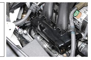
30. Reinstall the ECU to its mounting brackets.
