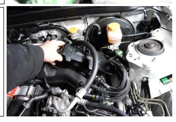
4. Locate the crossover fuel hose connection on the front of the LH fuel rail. The hose end fitting has a blue clip.
