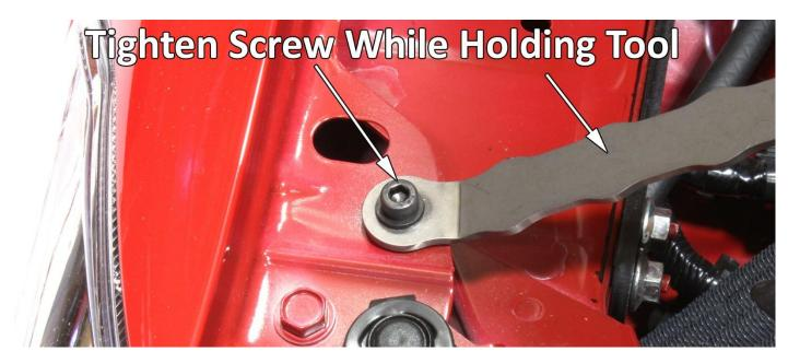
b. Continue to tighten M5 bolt (while holding the tool steady) until the turning force becomes harder, and/or stops. **NOTE: During this stage, the rivet nut is compressing and biting into the sheet metal from the inside.**
