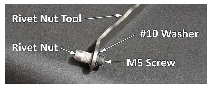
3. Install (1) #10 washer onto M5x16 socket cap screw, apply grease to threads and under head of bolt, install bolt through supplied tool, and install supplied M5 Rivet nut (with flange side facing tool). See picture above.
