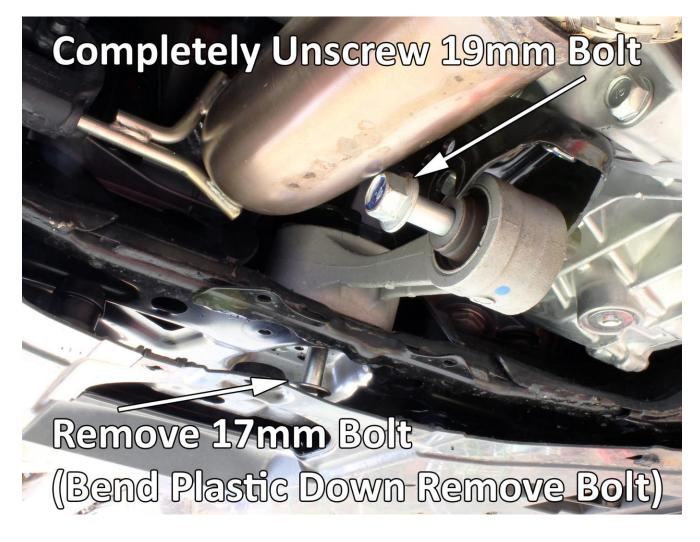
6. Remove rubber insert from motor mount as shown (on applicable models). **NOTE: This part is glued to the** center of the rear motor mount and may not pull off cleanly. If this happens, try to remove as much of it around the pivot as possible.
