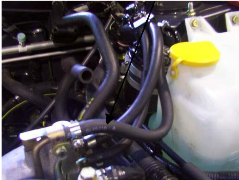
Illustration 4: Fuel Line Replaced to make room for Pipe # 2
