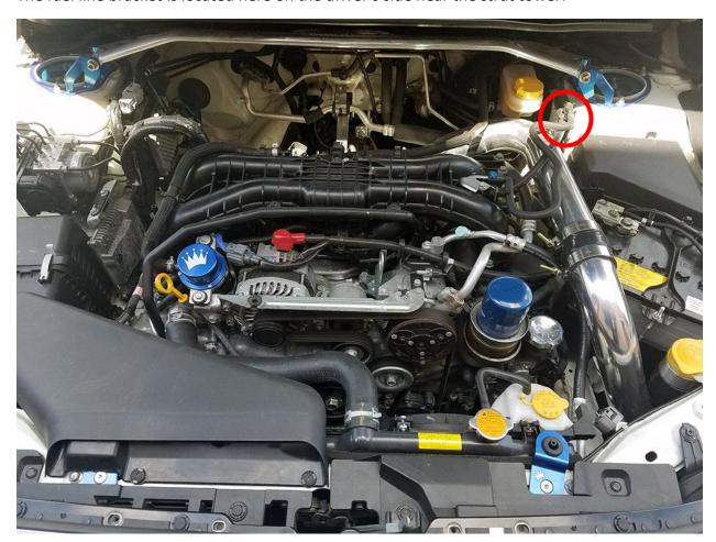
It is a two-piece bracket with two (2) bolts bolting the upper part of the bracket to the lower part of the bracket into the strut tower. To gain more clearance for the intercooler pipe to run under the fuel lines, remove both bolts, move the upper bracket "up" so that the lower bolt hole on the upper bracket aligns with the upper bolt hole on the lower bracket and screw them together.
