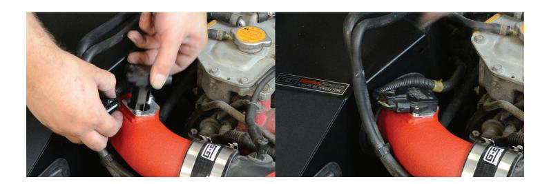
24. The OEM Airbox has two removable coolant hose clips. Use a needle nose pliers to remove the clips and set them aside.
