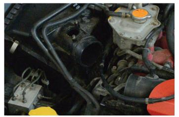
6. Unclip the lid fasteners from the airbox and remove the top so you can see the filter.
