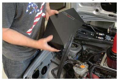
15. Take the last piece of bulb gasket and install it on the top facing edge using the same technique as you did for the other pieces.
