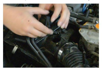
4. Using a flat head screwdriver, loosen the two OEM hose clamps on the stock intake elbow.
