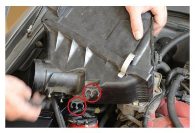
25. Take the clips and press them into the two holes on the side of the GrimmSpeed Heatshield.
