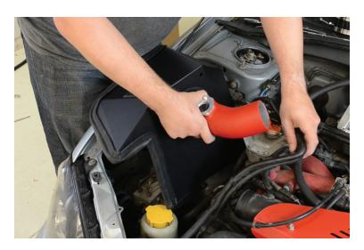
20. Your kit comes with two new 13mm bolts. Thread these with your fingers to hold everything in place. When re-installing the ground wire and bolt make sure to do it in the correct order... Chassis > Washer > Groundwire > Heatshield > Bolt.
