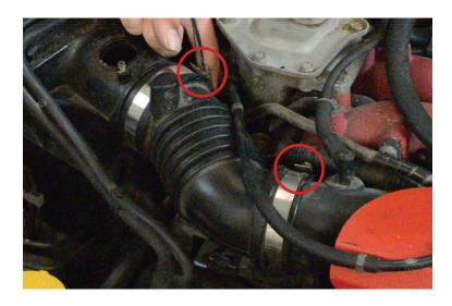
5. With the clamps loose you can pull the elbow off and set it aside.
