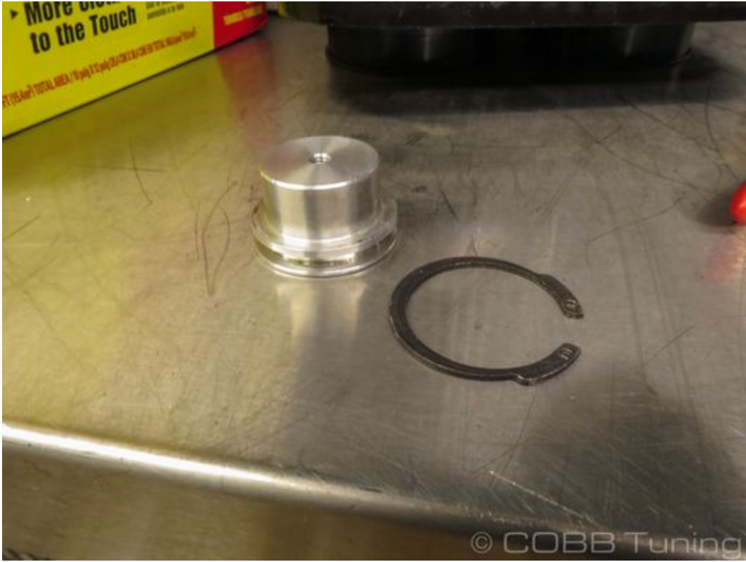
6. Now lubricate the o-ring with the provided lubricant and install it onto the sound suppressor.
