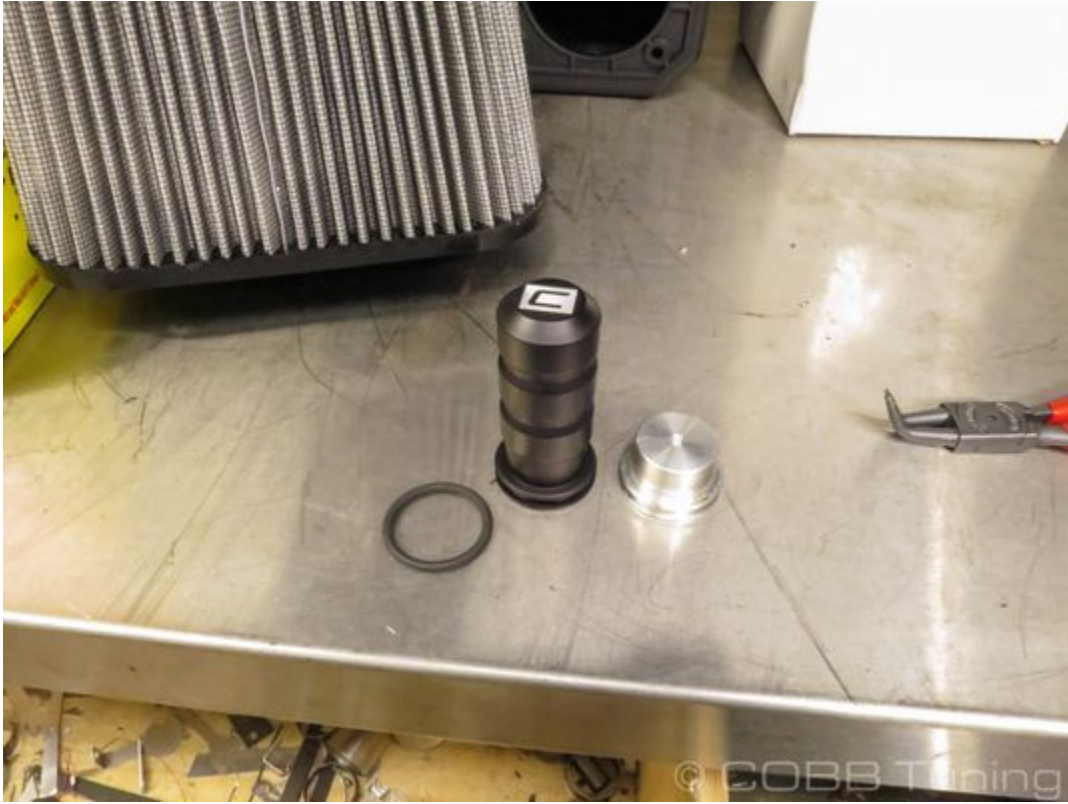
6. Now lubricate the o-ring with the provided lubricant and install it onto the sound suppressor.
