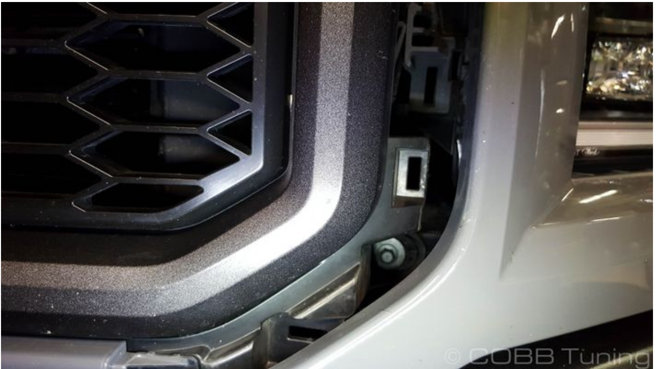
6. Remove the three clips on either side holding the rubber radiator shroud in place on the grille shroud.
