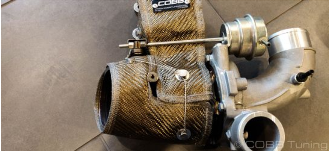
5. Here are some additional pictures that can give you a better idea of how to route the wire wrapping cleanly.
