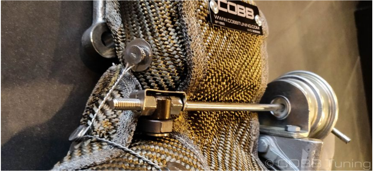
5. Here are some additional pictures that can give you a better idea of how to route the wire wrapping cleanly.
