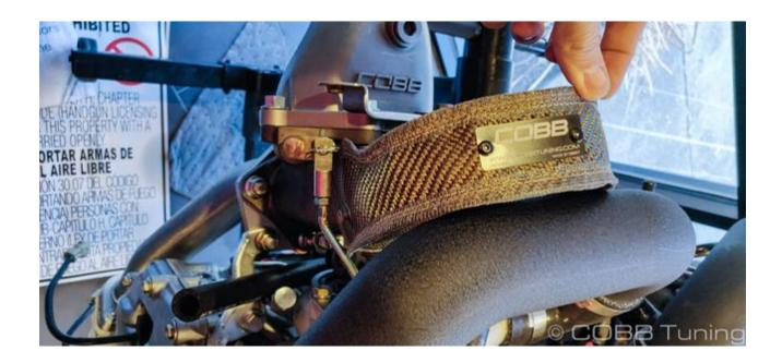
3. Now tuck the other side down around the turbo and under the bracket.
