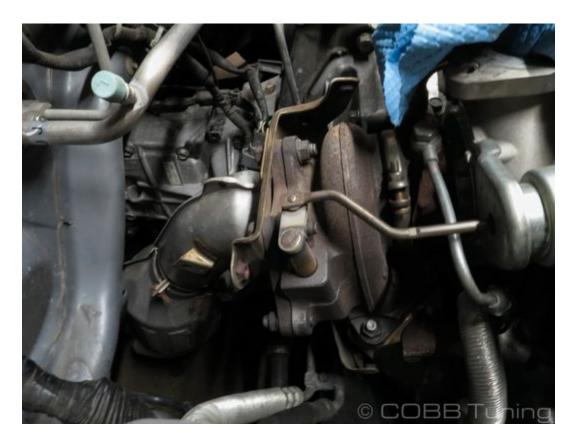
5. Now is a good time to check out the heat shield bracket as the factory units are quite prone to cracking and damage. Replace yours as needed.
