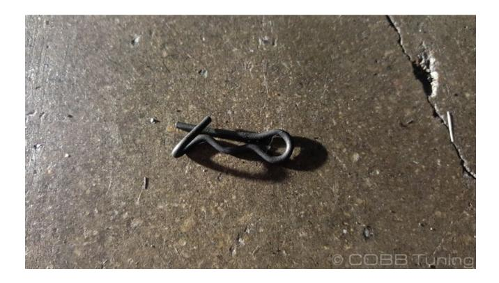
10. Pull out the retainer holding the cable in place.
