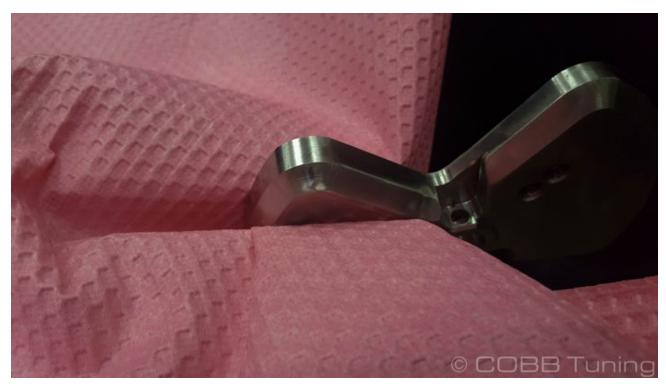
16. Tap the old pin in part way but not far enoug that it will stick into the bore where you'll install it onto the transmission.
