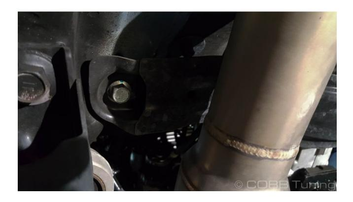
5. Undo the two central bolts going upwards onto the transmission mount.
