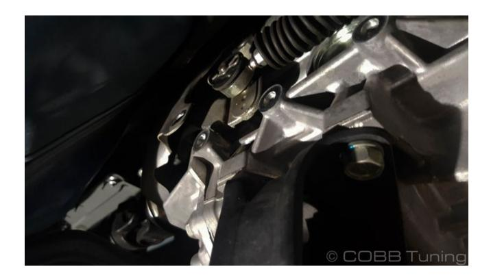
9. Remove the clip holding the cable in place and set it with the washer somewhere safe.
