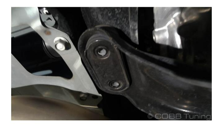
7. Remove the two 12mm bolts holding the long cable cover in place.
