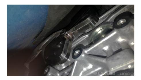
18. Add a small about of loctite to the pivot pin, then install it into the desired position using a 13mm wrench. The outer position will reduce the shift more than the inner one.
