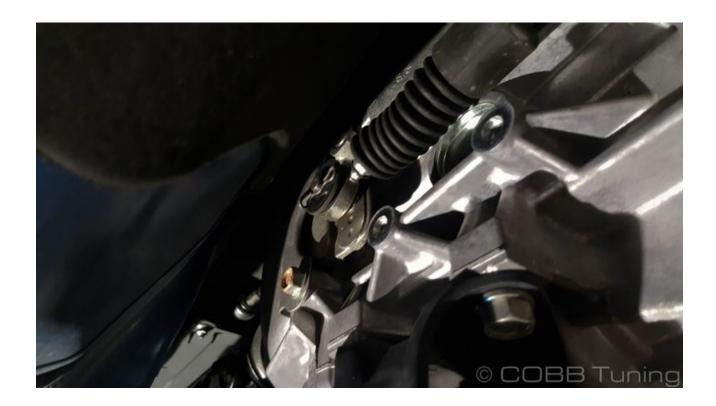
8. Remove the two easy to get to bolts on the passenger's side (right) and rear of the transmission. You should be able to slide it up and out of the way. You may need to loosen the top bolt to get it to slide if yours was installed tightly.
