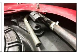
45. Safely lift and secure the vehicle. Find the fuel filter just left of the transmission.
