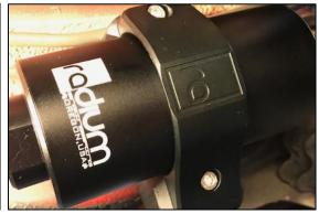
61. Using a 10mm socket wrench, remove the M6 bolt that secures the brake line adapter junction point shown.
