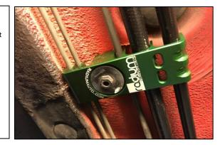
70. Just in front of the LH half shaft, the OEM hard lines make tight bends. For optimal fuel flow, the replacement fuel lines will bypass this potential restriction.
