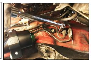
62. Relocate and secure the electrical ground wire ring terminal to the mounting boss, as shown.
