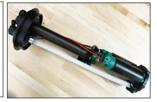
23. If not installed already, secure the Radium fuel sensor mount to the rear-most area of the triple pump block. Two of the bolts from the triple pump block will first need to be removed with a 3mm Allen wrench. Referencing the picture at the right, note the "REAR" engraving on the fuel top hat and the 2 bolts on the "rear" of the triple pump block.
