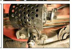
47. Using a 10mm socket wrench, remove the 2 bolts that secure the fuel filter to the fuel filter mount.
