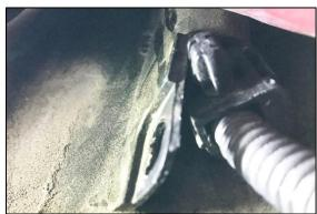
36. From above, dislodge the connector tabs and flip up. Cut all wires as close to the connector as possible. Remove some of the electrical tape and strip the wire insulation back  $\mathcal{K}''$ , as shown.
