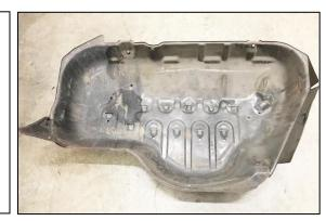
33. Using 10mm wrenches, remove the exhaust muffler shield. This piece is held in by 3 bolts.
