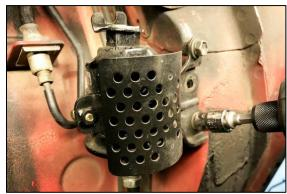
48. Using a 10mm socket wrench, remove the 2 bolts that secure the fuel filter mount to the chassis.
