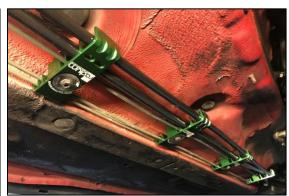
73. After tightening all related fittings, secure the fuel filter clamp using a 4mm Allen hex wrench. Notice how the filter is slide upwards inside the clamp to add ground clearance.
