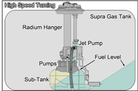
21. If using 1 or 2 fuel pumps or if sequentially staging 3 pumps, use a 2mm Allen wrench and install the jet pump retainer bracket to the top portion of the filter screen with the provided screw. To secure the jet pump return tube, insert the end into the retainer bracket, as shown. These 2 steps will already be done if the fuel hanger was purchased with fuel pumps included.
