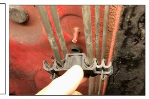
55. In one piece, pull the fuel feed line out of the vehicle. This will include everything from the fuel pump hanger banjo soft line to the fuel filter inlet inverted flare hard line, as shown.
