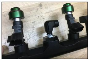
78. NPT threaded fittings should first be tightened finger tight. Then, using a wrench, add another 1.5 to 3 turns until fully tight and pointing straight up (same direction as the injector electrical connections).
