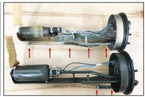
6. Only 2 parts will be reused from the OEM Toyota unit (gasket and sensors).
