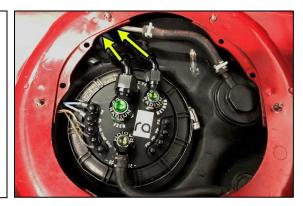
67. For this plumbing kit, the fuel pressure regulator (not included) must have a 6AN male return port. Radium Engineering recommends, DMR P/N: 20-0223-0X which can connect directly to the rear port of the Radium fuel rail. Line up the long return hose to the FPR and cut to length.
