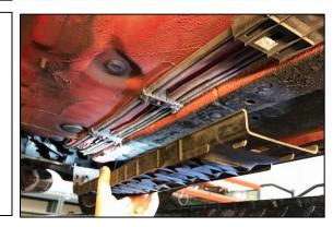
53. Using a 10mm socket wrench, remove the last plastic cover that is located to the left rear of the differential near the muffler.
