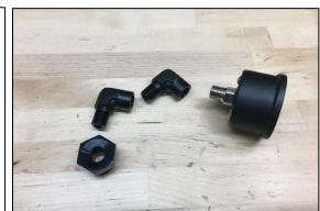
76. Install the 14-0119 into the rear most bottom port of the fuel rail as shown. Lubricate the O-ring with oil and tighten.
