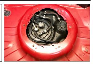
2. To depressurize the fuel system, first squeeze the tab and unplug the gray wiring connector on top of the pump housing (shown).
