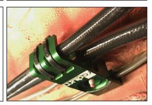
72. NOTE: the rearmost retainer will not require zip ties as the retainer touches the floorboard.
