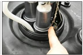
29. Readjust vertically and slowly lower the fuel hanger assembly downwards.
