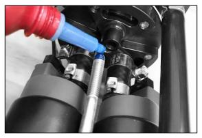
18. If installing 1 or 2 fuel pumps, screw in the bolt (shown red) with a 10mm socket wrench just enough before the filter assembly becomes crooked. Do NOT tighten! Use the included filter support bracket (shown blue) and the screws (shown yellow) to keep the assembly straight.
