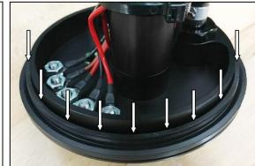
26. To install into the gas tank, the fuel level float must enter the gas tank first.
