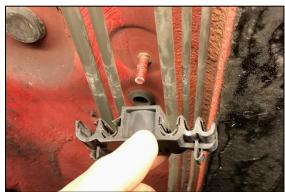
8. Note: There are a few different types of hard line retainers in the MKIV Toyota Supra. Some are shorter than others. For instance, the JZA80 chassis has raised M6 nuts in some locations.
