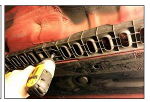
4. Pry the locking tabs to release the plastic hard line covers.
