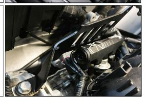
5. Using a 4mm Allen hex wrench and 10mm socket wrench, lineup the ECU and secure the top and front holes using the provided M6 button head screws and nuts.
