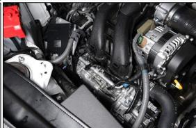
4. Set the new Radium ECU bracket in place. Using a 12mm socket wrench, secure using the two OEM M8 bolts.
