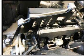
5. The ECU is chassis grounded through the engine using the bottom OEM mounting bolt. If this connection is forgot, the engine will not run. Secure with a 10mm socket wrench.
