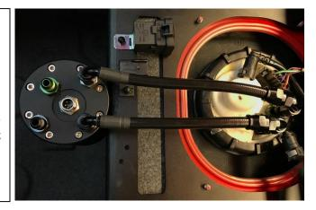
9. Find the 2 identical PTFE hoses that have straight and 90 degree fittings on the ends. Install the green Radium SAE male adapter fittings into the straight ends using 5/8" and 11/16" non-marring wrenches, as shown.
