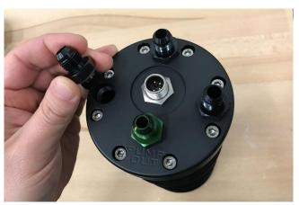
4. Remove the eight M5 bolts on the top plate of the fuel surge tank (FST) using a 4mm Allen hex wrench.
