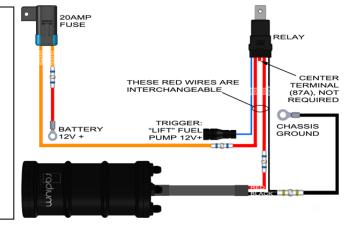
15. Note the different locations of the included solder butt connectors in the wiring schematic diagram above. There are 4 in total. The yellow solder butt connector is larger than the blue solder butt connectors.
