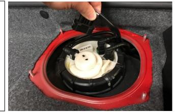
2. Temporarily install the large Radium mounting bracket attaching it to the 4 fuel pump access studs.
