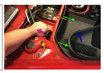
12. Drill two 1/8" holes through the rubber grommet. Be sure to stay clear of the existing wires that pass-through! These drilled holes will permit a weather tight seal for the fuel pump power wires. Insert the included red and black wires through the grommet, as shown.
