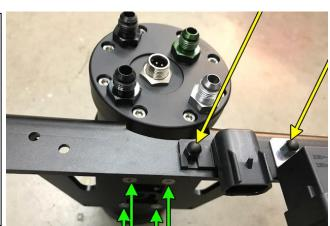
6. Place the large Radium mount assembly on the four OEM studs.
