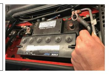
20. Lastly, place the Radium fuel pump module access cover onto the 4 studs. Using a 10mm socket wrench, install the 4 OEM acorn nuts (no OEM washers required).
