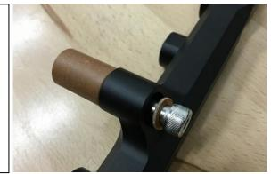
6. Place the fuel rail on the lower intake manifold. If using the OEM Nissan RB25DET manifold, there is a chance the phenolic spacers may create a slight interference. This is normal and the severity will depend on the machining in the casting. As shown, grinding is typically not necessary. NOTE: This will not be the case with aftermarket intake manifolds.
