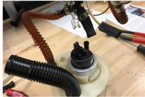
12. Pry the tabs around the upper sides of the basket to release the top portion with the fuel pump.
