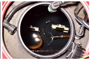
10. Pull the convoluted fuel return hose out of the top of the basket hole and set aside. It will be reinstalled later.
