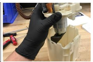
13. The fuel pump can now be separated from the assembly.
