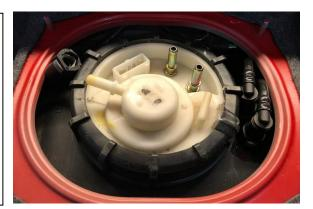
4. Use a white paint marker and draw a ½" straight line from the white plastic fuel hanger top through to the fuel tank lid threads. This allows a reference of how the fuel pump hanger is orientated so the level sender (in particular) is clocked properly when reinstalling.
