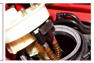
6. Carefully remove the level sender portion of the fuel hanger from the vehicle.
