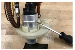
14. First, slide the Radium sleeve over the new pump. Insert the included worm drive clamp into the recess. For Walbro F90000262/274 pumps, fully seat the sleeve until it bottoms out. For all other pumps, the top of the sleeve and pump should be flush for proper positioning height. Secure using a 1/4" socket.
