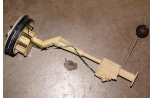
7. The next step is to remove both venturi jet pump arms from the fuel basket.
