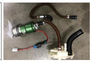
15. To fit the fuel pump back into the OEM plastic fuel pump cradle, first insert the sock filter. Next, slide the fuel pump down until the Radium sleeve's ring engages and fully seats into the OEM plastic fuel pump cradle.
