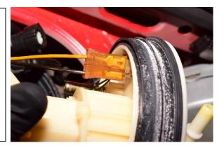
5. To release the factory quick disconnect fuel tubes on the underside of the fuel top, first remove the black plastic tab by pulling away (outwardly).
