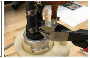
11. Pull the Y-fitting hose assembly off the fuel pump barb.
