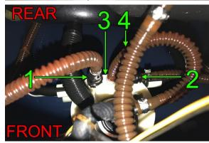
8. Pull the venturi jet pump arms outwards to release.
