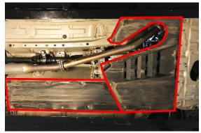
24. Find the mounting bracket and three M8 button head screws in the kit. Using a 5mm Allen hex wrench, secure the bracket to LH tunnel over the hard lines near the transmission.
