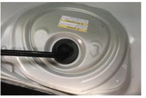
35. The Radium FPR does NOT come preset to a specific pressure. To adjust, loosen the jam nut with a 3/8" wrench. Using a 3/32" Allen hex wrench, spin the set screw clockwise to increase pressure and counterclockwise to decrease fuel pressure. Use the pressure gauge as a reference.
