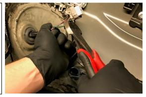
21. Cut two  $\chi''$  pieces of the small diameter shrink tube. Insert onto each sensor wire (two small gauge wires). Next, crimp on a small gauge (AWG) ring terminal to each wire. Slide the shrink tube over the crimped section of the ring terminal and shrink into place with a heat gun. Extra parts may be present in the kit and can be used as spares.
