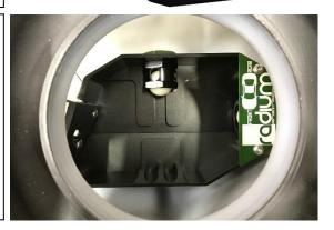
15. Find the OEM rubber gasket that was previously removed from the OEM module. Fully seat the gasket onto the fuel tank, as shown. Make sure it stays seated throughout the rest of the installation process.
