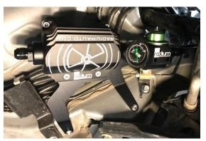
30. To make room near the fuel pump hanger, the rear most OEM fuel lines should be removed.
