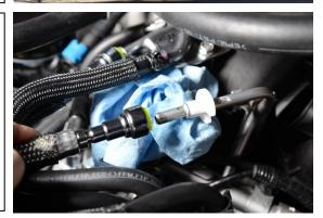
33. The two -6AN fuel lines from the Radium FPR are identical and cannot be criss-crossed. They can be connected to either the HPFP line or the port injection fuel line.
