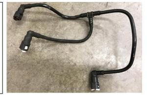
31. Find the provided 3/8" fuel hose and two -6AN PushLok hose ends. Lubricate the straight hose end barbs and fully insert it into one side of the 3/8" fuel hose. Loosely route the hose between the outer front side of the gas tank and the foot well sheet metal. This may require access from the cabin and underneath the car. Route the -8AN PTFE hose in the same fashion.
