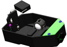
14. Observe the orientation of the collector box in the picture at right. The fuel level sender should be positioned at the RH side of the gas tank. The collector box should naturally fall into place with the contours of the gas tank floor. The green baffle plate should be indicating the correct orientation with respect to the vehicle.
