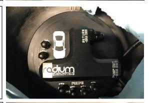
18. The top plate and gasket should be flush with the fuel tank lid area.
