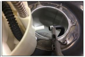
5. To remove the fuel level and fuel temperature sensors from the OEM fuel pump housing, first depress the thumb tab and unplug the 3-pin connector from underneath the top plate. Next, pry and pop the fuel temperature sensor probe out of the securing tabs.
