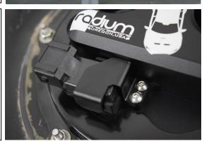
20. External Wiring: Cut off the OEM 5-pin fuel pump control module connector, as shown.
