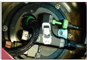
35. Torque the 5/16" SAE Male Fitting into either end of the PTFE hose included in the kit. If installing to a Radium fuel rail with a DMR installed onto the top port, make sure the 6AN male return fitting is pointing towards the left side of the vehicle. Loosely install the opposing hose end to the DMR's 6AN male fitting. NOTE: Hose routing will differ if installing onto a different brand pressure regulator.
