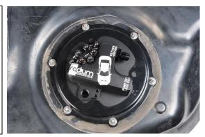
18. The top plate and gasket should be flush with the mounting ring.
