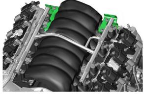
9. The 20-0232 fuel rail does not include plumbing. NOTE: Early LS1 engines (97-99) will require an aftermarket FPR to replace the regulator on the OEM rail.
