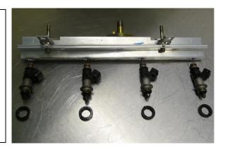
10. Install the OEM FPR to the Radium fuel rail using the OEM hex head bolts. Inspect the O-ring for damage or tears. Replace if necessary. The FPR screen from the OEM rail will not be reused.
