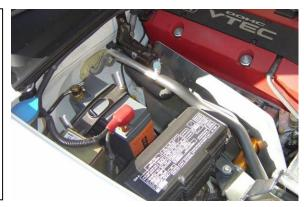
3. Using a pair of pliers, release the OEM spring clamps from the PCV valve and crankcase breather hoses found on the valve cover. Carefully pull the hose off the PCV valve barb.
