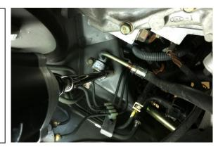
16. Remove and discard the Honda OEM soft rubber hose (shown) from the vehicle.
