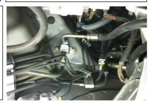
15. Using a 10mm socket wrench and extension, remove the two M6 bolts that secure the fuel feed line clamp to the chassis, as shown. These will not be reused.
