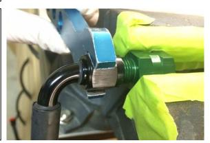
18. From underneath the vehicle, mate the inverted flare fittings. Route the PTFE hose upwards staying clear of hot and/or moving parts. Secure to the -6AN male fitting on the top port of the fuel rail.
