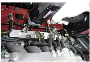
8. Unclip the fuel injector wiring harness from the 2 stays. Unplug the fuel injector connectors and carefully pull the fuel rail out of the vehicle. Have a rag handy as there will be excess fuel still remaining in the fuel rail.
