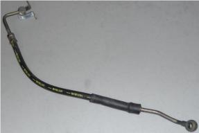
17. Find the female inverted flare to -6AN male adapter fitting in the kit. Screw and secure it to the Radium PTFE hose.
