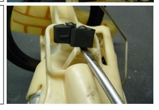
10. Next, the plastic pump holder will need to be separated from the BMW fuel pump. First, take note of the clocking orientation of the plastic holder in respect to the fuel pump's outlet barb. Pull the tabs downward (as shown) to release the pump. NOTE: The holder will come out the bottom of the pump.
