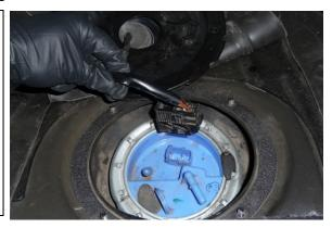
5. To release the factory quick disconnect feed line fitting, simply rotate the connector until both outer tabs can be accessed with a thumb and index finger.
