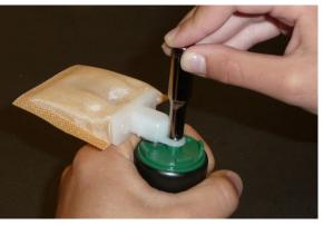
20. Position the new fuel pump assembly back into the BMW hanger. Reinstall the rubber isolation grommets from the previous steps.
