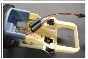
18. First, slide the billet sleeve into the BMW plastic holder. Next, slide the fuel pump into the billet sleeve.
