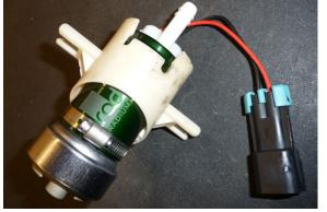
19. Locate the new fuel pump sock filter and the metal lock washer. Insert the sock onto the bottom of the pump. This installs only one way. NOTE: filter sock may differ than picture.
