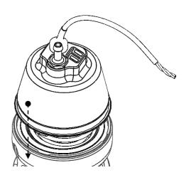
Ensure when assembling sensor cap onto BOV body that the wiring loom is not damaged or crushed. Please refer to "HOW TO CHANGE YOUR POWER PORT BOV SPRING" parts 3 thru 5 for reassembly of your Power Port BOV for accurate cap installation steps.
