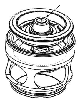
Using a 4mm allen key, undo the bolt at the centre of the diaphragm holding it to the valve stem. Wipe off any residue left behind on the valve stem.
