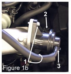
Replace the two bolts, recirc and vacuum hoses and clamps.
