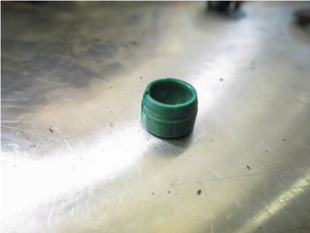
13. With the cup free pop it in the lower skinnier portion of the COBB shifter cable bushing.
