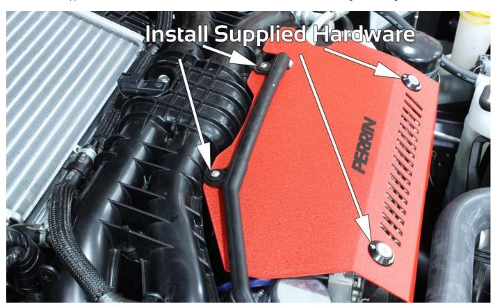
10. Adjust plastic hose and belt cover until it is lined up with front of car. Tighten 10-32 screws until hand tight. **NOTE:** As the screws are tightened up, the rubber well nut compresses and grabs back side of hole in manifold creating a secure mount. It is important
