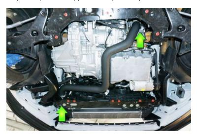
7. Insert and tighten the M6x25 flanged hex bolt to 12 FT/LB to the transmission stud location. Use a 10mm socket to tighten the stud bolt.
