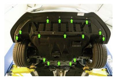
2. Remove front under tray (plastic). There are (6) Torx 27 screws and (7) additional screws. There is one screw in each wheel well that will need to be removed.
