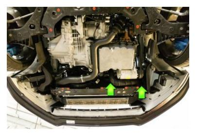
5. Remove the OEM hot side piping by loosening the clamp at the intercooler and the other clamp at the turbo.
