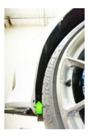
3. Remove the chassis brace on each side of the car. There is an inner 15mm bolt and an outer 18mm bolt on each brace.
