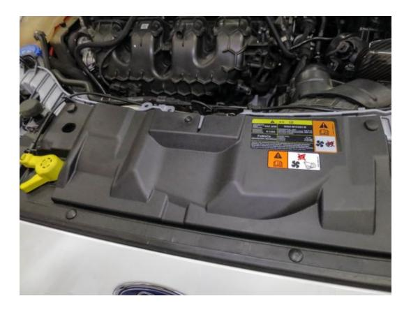
5. In the engine bay remove the cable for the hood release by lifting the cable up in order to release it from the holder, then moving the cable towards the handle to release pressure and allow you to pop the cable retainer out of the top.
