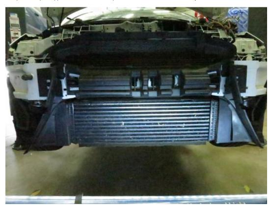
10. Remove the radiator cowling by squeezing the clips inside of the bumper support and unbolting the two T20 screws
