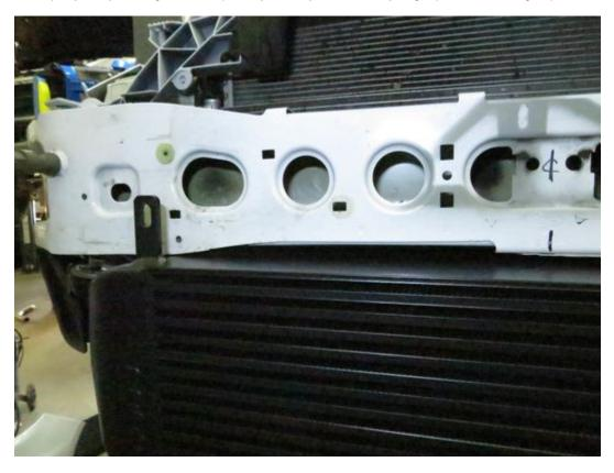
22. Assemble the bolts as shown. You'll use the M6x30mm bolts with a washer on either side of a rubber bumper, placing that between the intercooler mount and the bumper, with a washer by itself on the inside of the bumper beam and a 20mm width washer on the outside.
