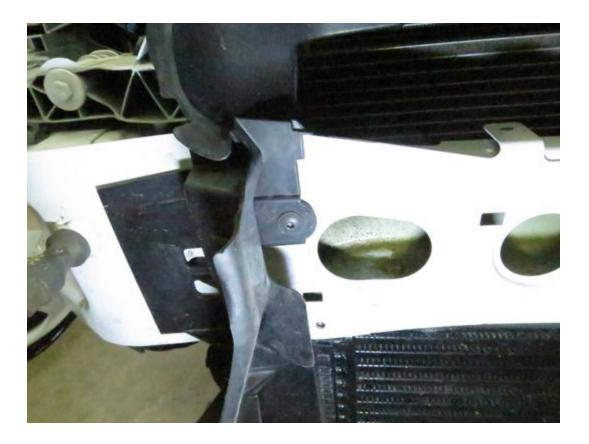
11. Take out the side covers, they should pop out simply with some minor wiggling and you can wait until after the core is removed to remove the driver's side if it won't come out easily.
