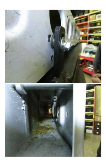
23. Now do the same thing with the lower mounts, using a rubber washer sandwich on either side of the vehicle side support and a washer under the bolt head going down through the entire assembly.
