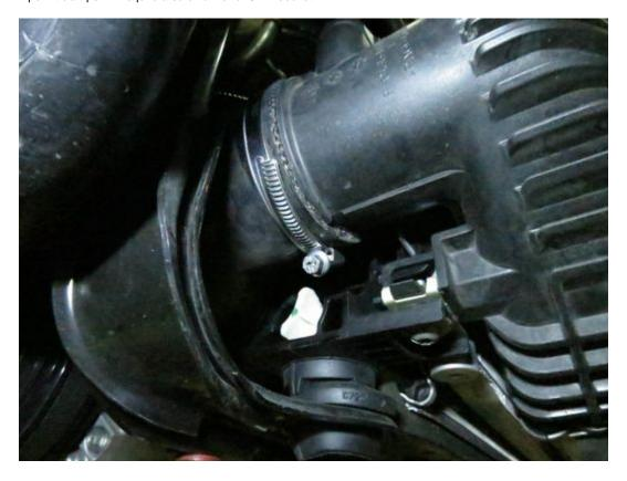
14. Undo the two T30 screws on the bottom of the intercooler mounting it to the car.
