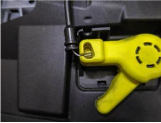
6. Now pull outward on the corners of the bumper in order to release them from the clips under the headlight. Be careful not to scratch them, applying painters tape to the edge of each fender to prevent scratches as things move around and as you remove the rest of the bumper.
