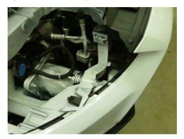
8. Once the bumper is loose, disconnect the fog light wiring on the driver's side. Once done set the bumper somewhere safe and out of the way to prevent damage
