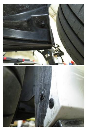
4. In the engine bay remove the two trim clips and four T27 bolts holding the upper trim piece in place.
