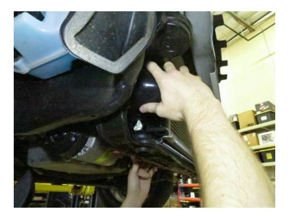
21. Now line up the core with the square holes in the bumper. Using a jack of some kind to support it will make things infinitely easier as the core is pretty heavy. Having a friend help steady it while you attach everything in place can be a big help.
