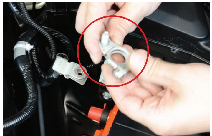
22. When you pull the terminal apart, it will separate into 3 pieces. Flip the terminal around so it is facing the other direction.
