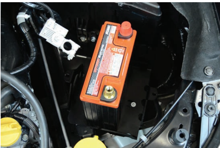
15. Install the included terminals on to your PC680 battery with a 12mm allen. Make sure to use the correct terminal for the positive and negative sides of the battery.
