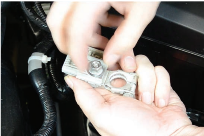
21. Undo the 10mm bolt on the positive side of the terminal.
