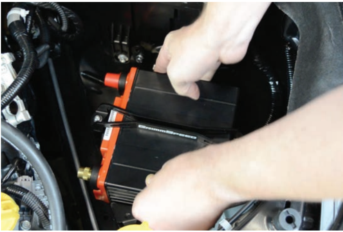
19. Give the battery tray a shake to make sure everything is tight and securely in place.
