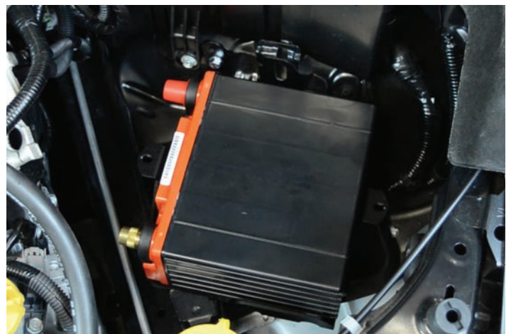
16. Lay the battery down on its side. Terminals facing up.
