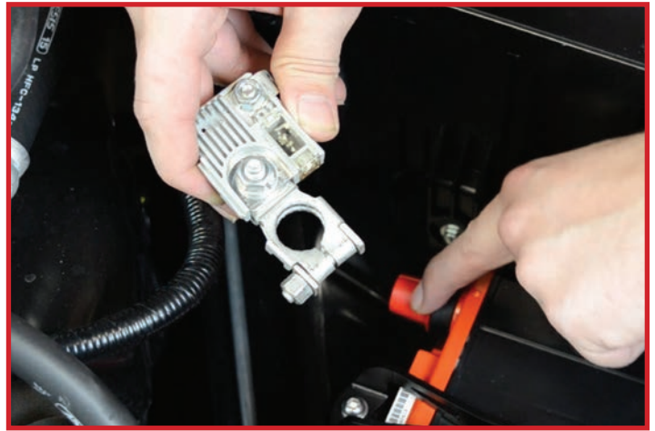
20. The OEM Terminal on your WRX/STI is tapered and won't fit properly on your PC680 Battery unless you modify it.
