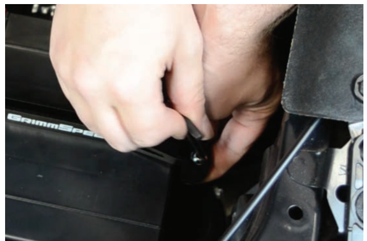
18. Thread the included nut on to each bolt. Then, using your 10mm wrench and 3mm allen wrench tighten the bracket on each side evenly.
