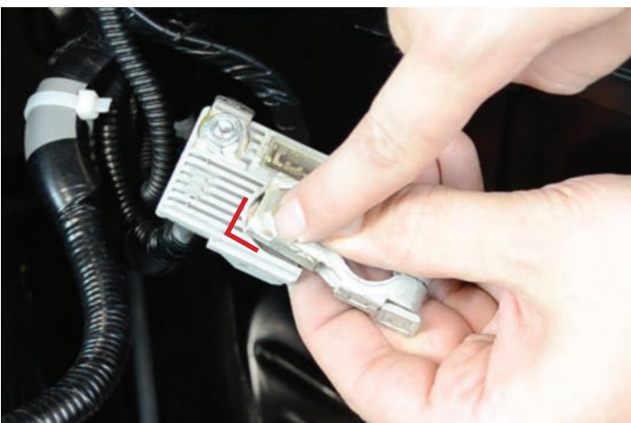
23. If you are installing this kit on a 2015+ WRX or STI you will notice that the terminal can not be flipped due to the 90 degree edges.
