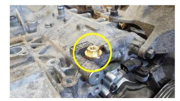
5. Attach the pressure pot line to engine with the appropriate metric to NPT adapter mentioned in Step 4.
