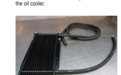
» Route the 24" section of hose from the bottom of the cooler to the top of the oil reservoir.
