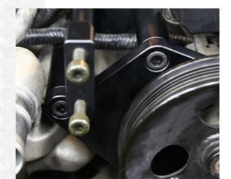
» Line up the holes in the power steering pulley with the three mounting bolt holes on the pump and then line up the pump bracket.
