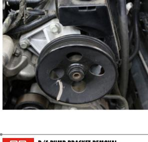
» Rotate the power steering pulley until the holes in the pulley line up with the three pump mounting bolts.
