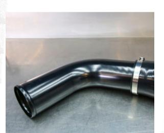
Install the end of the pipe, without a coupler, into the upper passenger-side charge pipe coupler. Once installed, rotate the MAF pipe so that it lines up with the throttle body.
