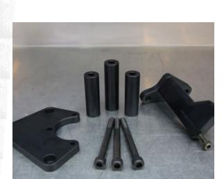
» Locate the supercharger mounting bracket(s) with power steering mount as shown.
