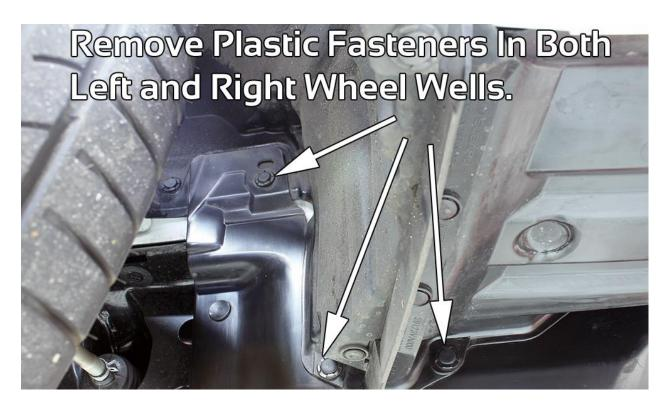
2. Using proper panel removal tool or flat head screw driver, locate and remove (7) plastic fasteners and (2) 12mm headed bolts from lower portion of splash guard. See picture below.
