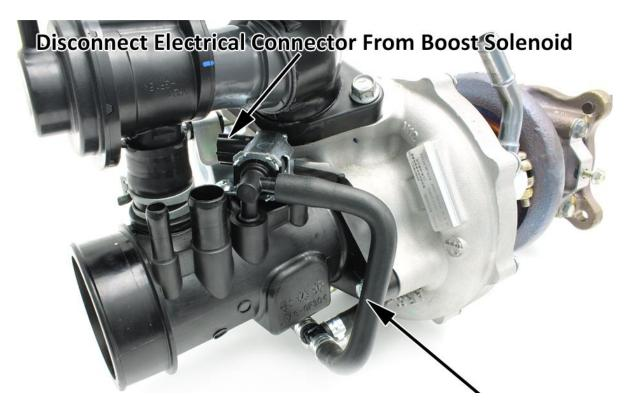
6. Locate vacuum hose coming off solenoid (see arrow in picture above), and remove from "tee" junction on lower side of turbo.
