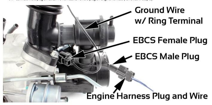
18. Locate engine ground on right side engine head. Remove 10mm bolt (with OEM engine ground still on bolt) and place ring terminal from EBCS Pro harness on bolt, then reinstall back to head. **NOTE: Both the OEM and EBCS Pro harnesses will be grounded using same bolt.**
