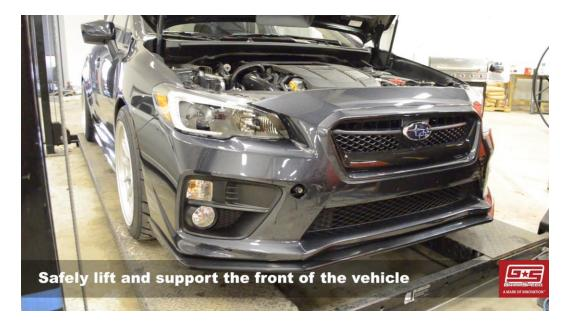
2. Next, remove the factory splash guard. You'll need to remove four pop clips surrounding the skid plate, three clips on each side of the car and then three clips along the leading edge of the splash guard. Lastly, use a 12mm socket to remove the two bolts securing the front of the splash guard.
