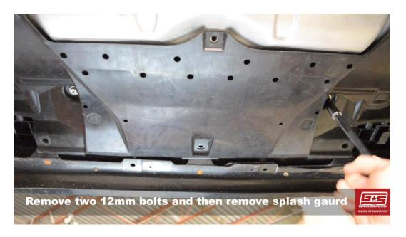
3. Next, remove the factory skid plate by removing the four 12mm bolts securing it. Be sure to support its weight when removing the final bolts.
