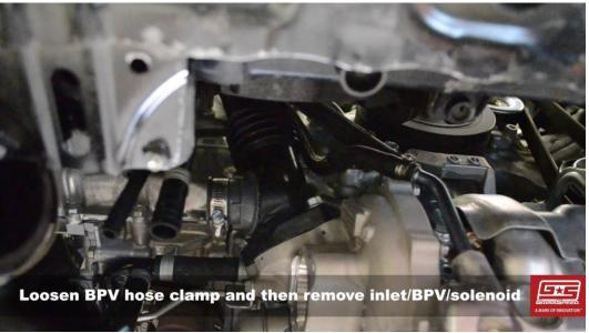
10. Remove the two Philips screws securing the factory boost control solenoid to the turbo inlet. You may need to twist the bypass valve out of the way to get access to one of the screws, just remember to twist it back later. Once the two screws have been removed, remove the factory solenoid and set it aside.
