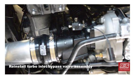
14. Reach behind the turbo and connect the GrimmSpeed solenoid to the factory wiring harness.
