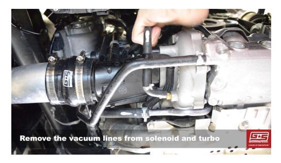
5. Disconnect the two large hoses that are attached to the turbo inlet. One has a spring clamp that you'll need to move using your pliers. At this time, you can also disconnect the small vacuum hose that's attached to the bypass valve. No clamp here, so just tug on it.
