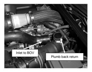
3) Remove the standard vacuum line and replace it with the provided silicone vacuum tube. Secure the end with a hose clamp
