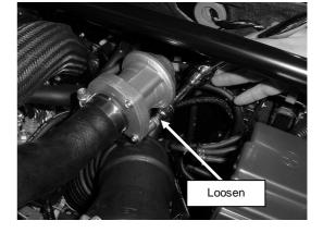
2) Remove the piping and vacuum line off the standard BOV
