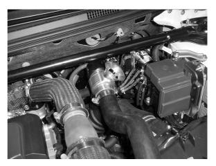
Note: The Dual port is supplied with a blanking plug for the vent to atmosphere side of the BOV to convert the BOV to full recirculation mode. Simply unscrew the trumpet and screw in the supplied blanking plug. Alternatively, the blanking plug can be used to convert the BOV into full vent to atmosphere mode by installing the blank onto the plumb back side. An additional 34mm hose blank (sold separately) is required to block off the plumb back hole in the intake pipe.
