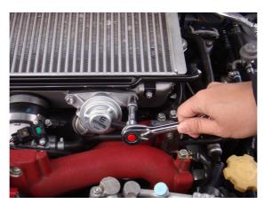
2. Using pliers, carefully clamp onto the spring clamp on the plumb back hose and pull the BOV off the hose. Then carefully remove the clamp completely.
