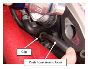
7. Secure the BOV onto the intercooler with the standard bolts and replace the vacuum line to the top of the BOV.
