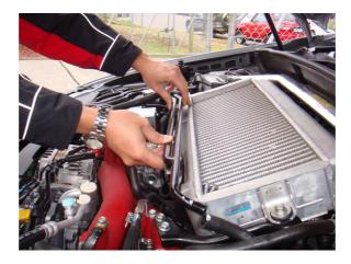
5. Using the provided ½" tee piece, connect the standard oil breather lines on the left hand side of the intercooler in the orientation shown in the picture below and run the provided ½" hose under the intercooler to the oil breather line on the other side of the intercooler, using the provided ½" straight joiner to join the rubber hose to the existing breather line on the right hand side.
