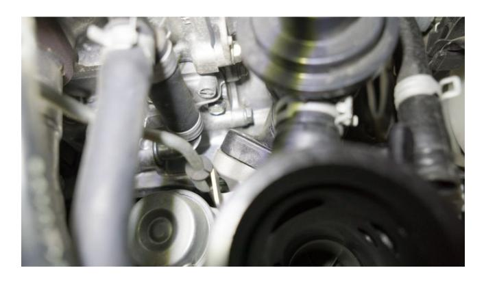
7. Applying a small amount of pressure, remove the BPV from the turbo inlet.
