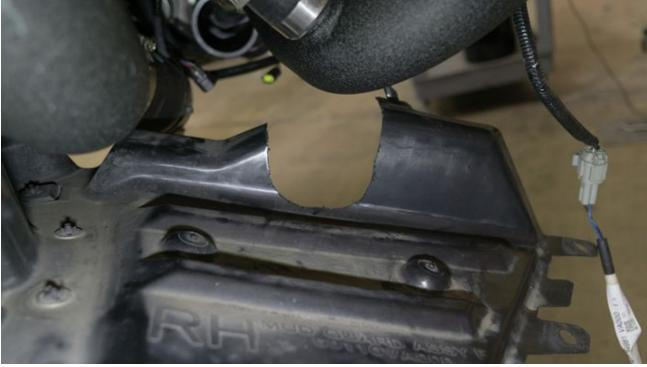
11. Release the breather hose by removing the (2) plastic Phillips head push pins.
