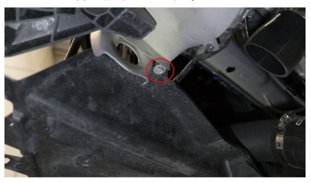
b. Secure the lower wheel well tray by screw (1) Phillips head screw on the driver side.
