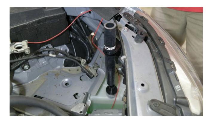
19. Install washer fill hose on reservoir spout adapter.
