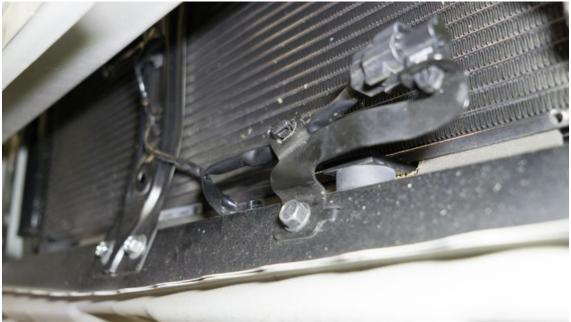
m. Remove the bumper beam by unbolting (8) 12mm bolts. There will be (4) on each side.
