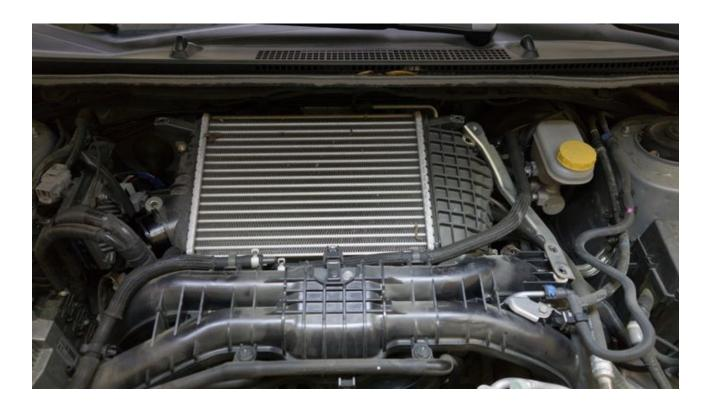
13. The TMIC should easily lift away from the motor.
