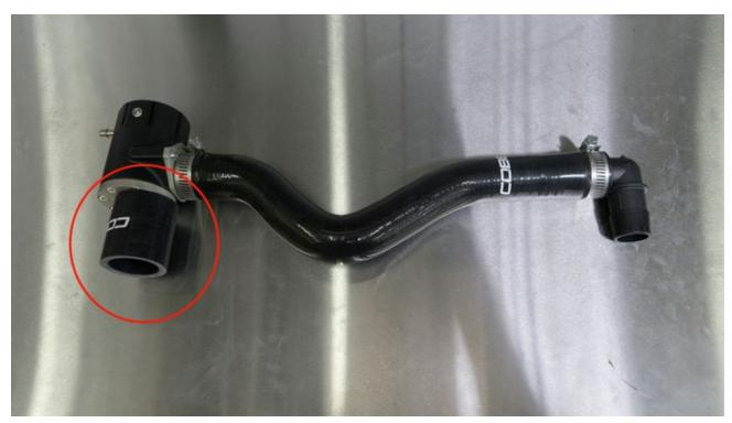
6. Attach a 3" - 2.5" silicone reducer to the intercooler using a #48 clamp.
