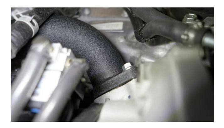
3. Attach the BPV recirculation silicone to the BPV using #16 clamp.
