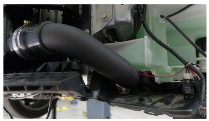
4. Attach a 2.5" silicone coupler to the lower intercooler piping using a #44 clamp.
