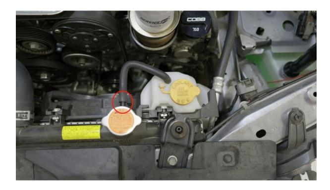
2. Release the retaining clip for the reservoir assembly.
