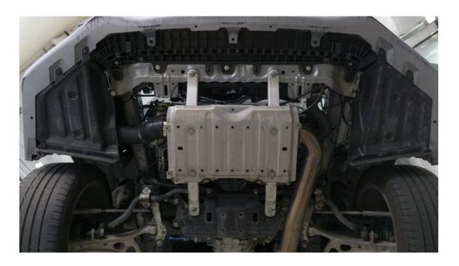
e. Remove the lower wheel well tray by unscrewing (1) Phillips head screw on the driver side.
