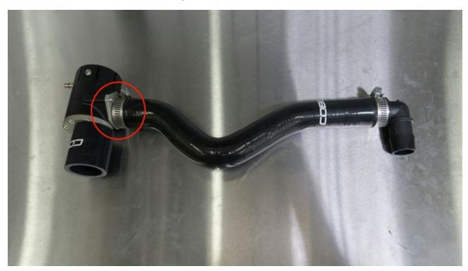
4. Attach the BPV recirculation silicone to the 1" 90 degree fitting using a #16 clamp.
