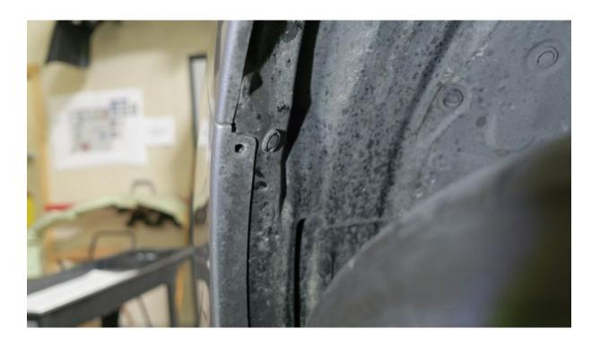
c. Release (1) push clip from the passenger side wheel well.
