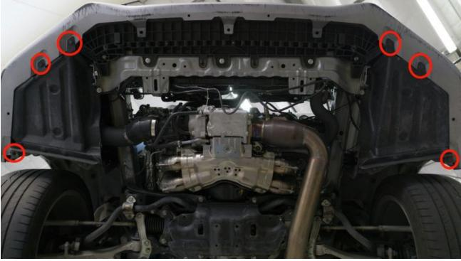
9. Install the skid plate by bolting (4) 12mm bolts.
