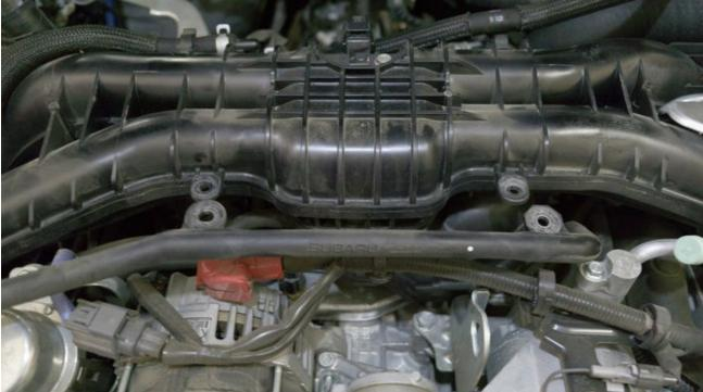
12. Cut the breather hose so it's in line with the adjacent hardline (helps to mark it with a silver Sharpie or similar).
