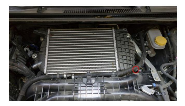
12. Remove (4) 12mm bolts holding the intercooler down.
