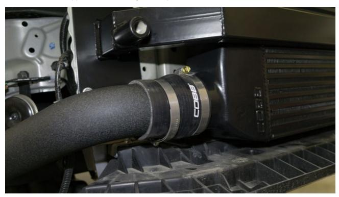
8. Attach the lower intercooler pipe to the BPV coupler using a #36 clamp.
