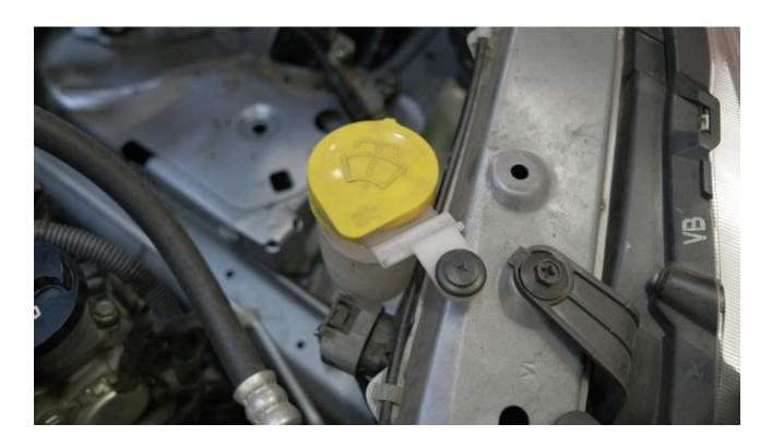
2. Twist and remove the reservoir spout head.
