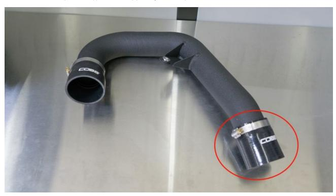
7. Attach a 2.75" - 2.5" silicone reducer to the upper intercooler pipe using a #44 clamp.
