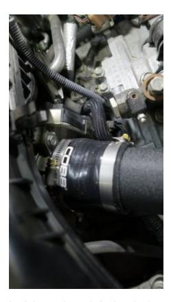
10. Attach the upper intercooler bracket using the provided M8x25 bolt.
