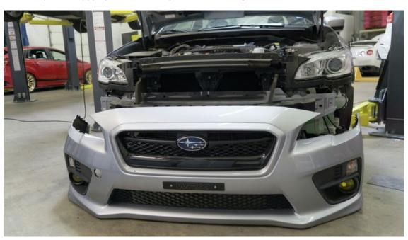
j. As you remove the bumper, be wary of the foglight connectors. You should have enough length in the harness to gently set the bumper down while you disconnect the harness.
