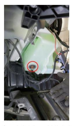
8. Remove the electrical harness clip holding it to the reservoir.
