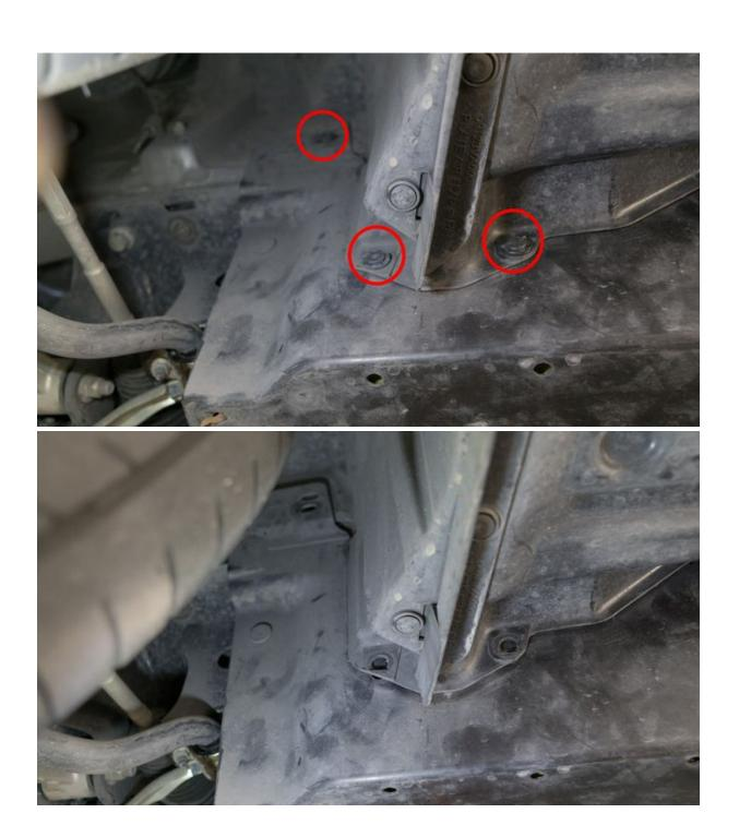
b. Release the (3) flathead push-clips from the driver wheel well.
