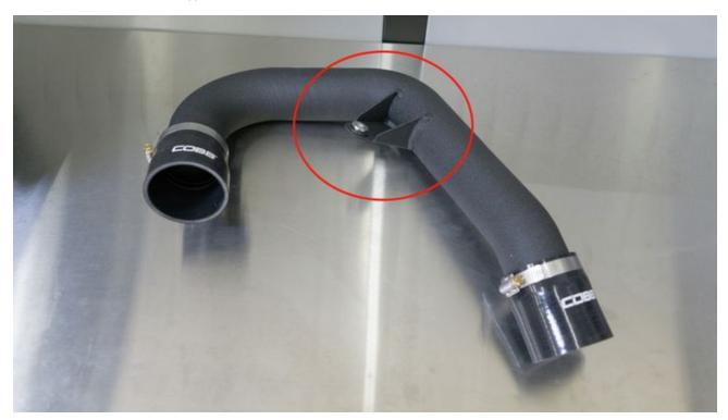
9. Attach the assembled upper intercooler pipe to the throttle body and middle intercooler piping. Use a #44 clamp on the side attaching to the middle intercooler piping and a #48 clamp on the side attaching to the throttle body.
