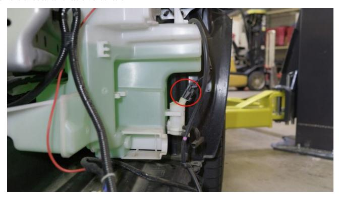
7. Remove the washer fluid level sensor.
