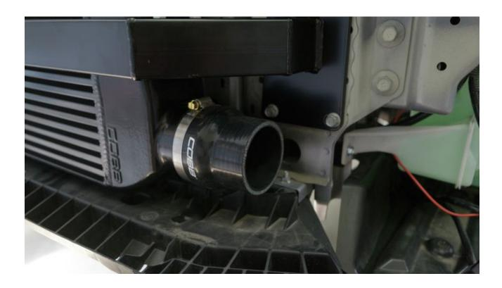
3. Attach the lower intercooler pipe using a #44 clamp.
