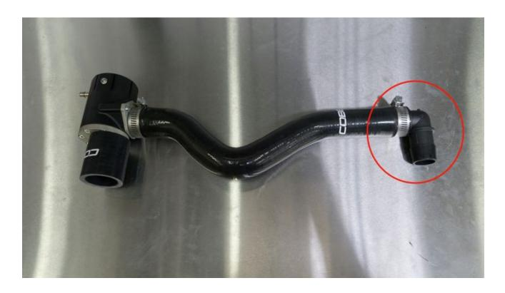
5. Attach the BPV coupler to the BPV using a #24 clamp.
