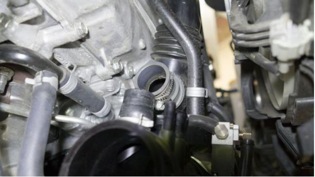
9. Loosen the clamp from the intercooler to hot pipe.
