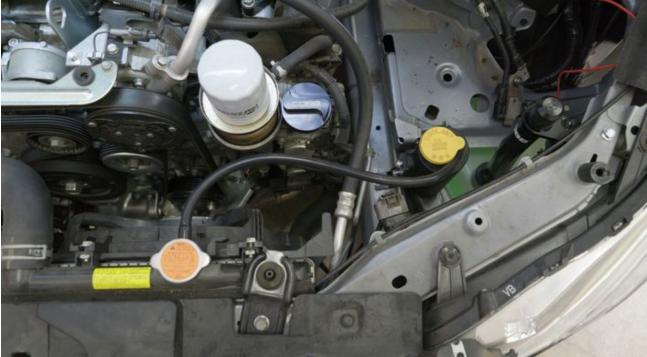
10. Fill the coolant reservoir with coolant until it's 1/2-3/4 full.
