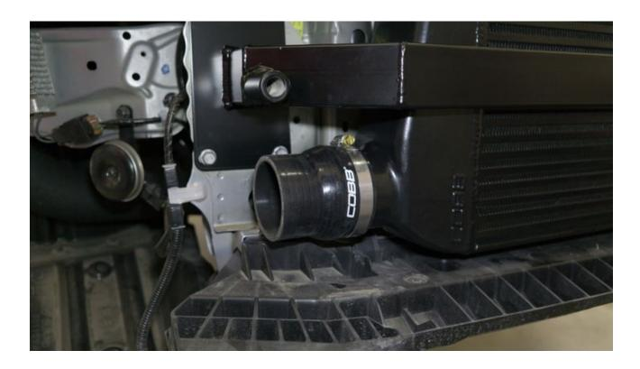
7. Attach the lower intercooler pipe to the intercooler using a #44 clamp.
