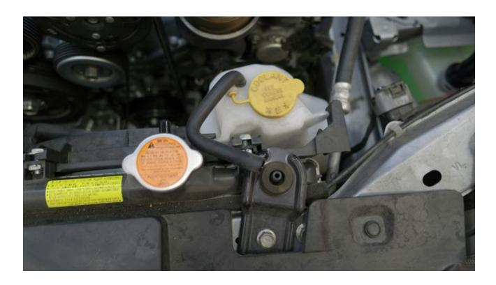
3. Remove the entire coolant reservoir assembly.
