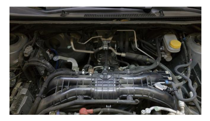
14. Loosen the 8mm clamp on the throttle body coupler and remove the coupler..
