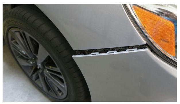
h. Release the bumper pressure clips on the driver side wheel arch by applying a small amount of outward pressure.
