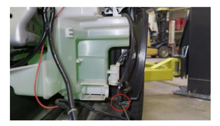
6. Remove the electrical harness for the fluid washer.
