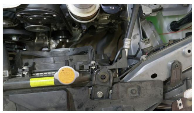
4. Attach the coolant reservoir bracket to the coolant reservoir using the provided (2) 6mm socket head cap screws with washers and (1) flange head bolt.
