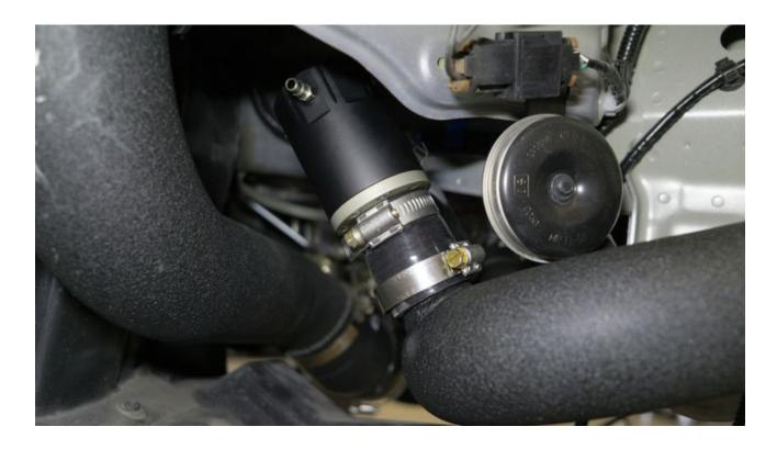
9. Attach the lower intercooler pipe to the upper intercooler pipe using a #36 clamp.
