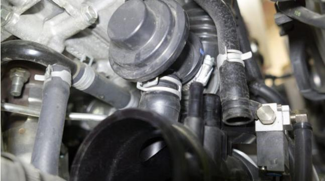
4. Remove the vacuum hose to the BPV.
