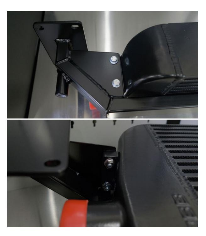
2. Install the bumper beam with the attached FMIC to the car. You will be using the factory (4) 8mm bolts with 12mm heads on each side.
