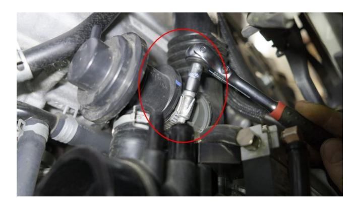
6. Remove (2) 12mm bolts on the factory hot pipe to turbo. You will need a 6" extension for one of the bolts.
