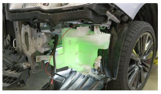
14. Clip the washer fluid level sensor back in.
