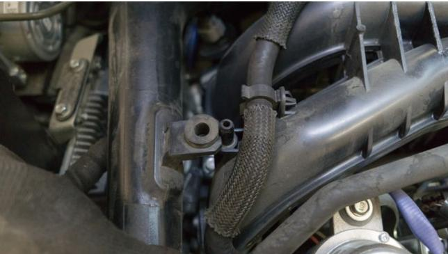
11. Loosen the 8mm clamp on the right hand side of the intercooler.
