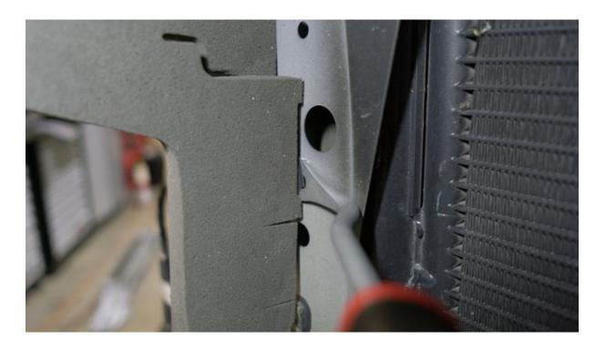
o. Flip the horn orientation as depicted. You will need unbolt (1) 12mm bolt and release the retainer clip. Once released, you will flip the horn around and when bolted back up, the bolt will be facing the engine bay.
