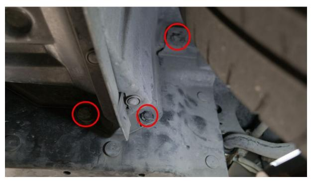
f. Insert the (3) flathead push-clips form the passenger wheel well.
