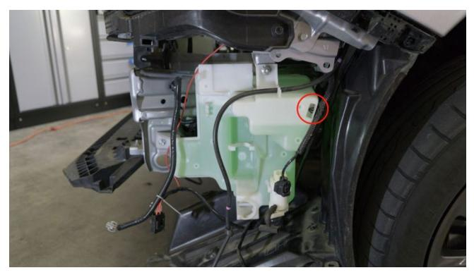
9. Using a 12" extension, remove (3) 10mm bolts holding the reservoir to the chassis.
