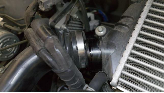
10. Remove the hot side pipe. Be cautious of the retainer clip near the intake manifold.
