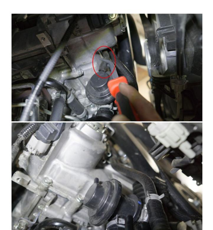
5. Loosen the BPV to factory hot pipe clamp.
