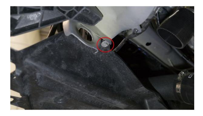
2. Remove the skid plate by unbolting (4) 12mm bolts.
