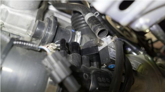
2. Loosen the intake silicone clamp to allow access to the BPV.
