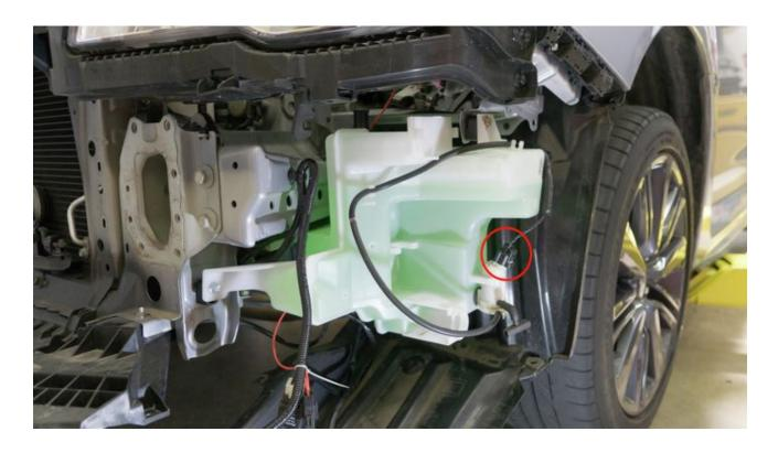
17. Install washer fill bracket using the provided (1) 6mm flange head bolt.
