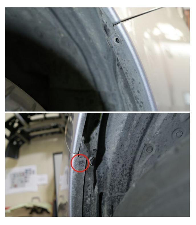
7. Insert (1) push clip on the passenger side wheel well.
