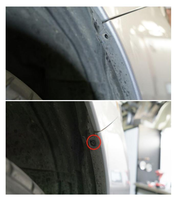
8. On the bottom of the bumper, insert the (6) push clips.
