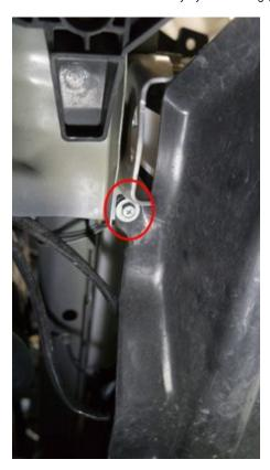
f. Remove the lower wheel well tray by unscrewing (1) Phillips head screw on the passenger side.
