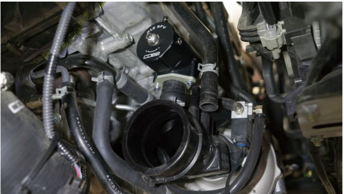
3. Cut approximately 25" of 6mm vacuum hose and connect the BPV to the reference line.
