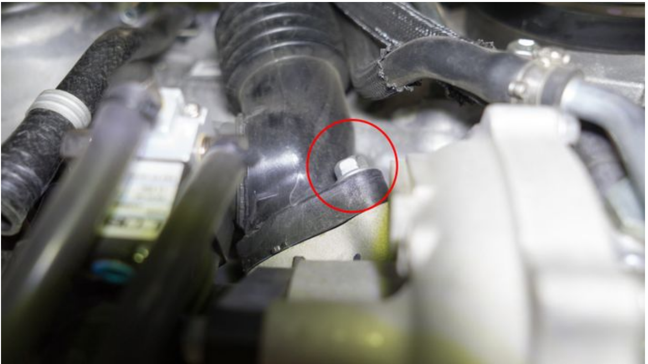
6. Remove (2) 12mm bolts on the factory hot pipe to turbo. You will need a 6" extension for one of the bolts.
