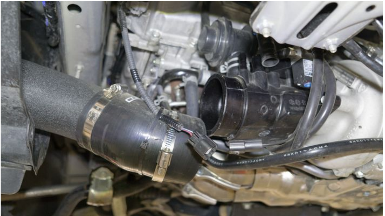
3. Loosen the BPV to factory turbo inlet clamp.
