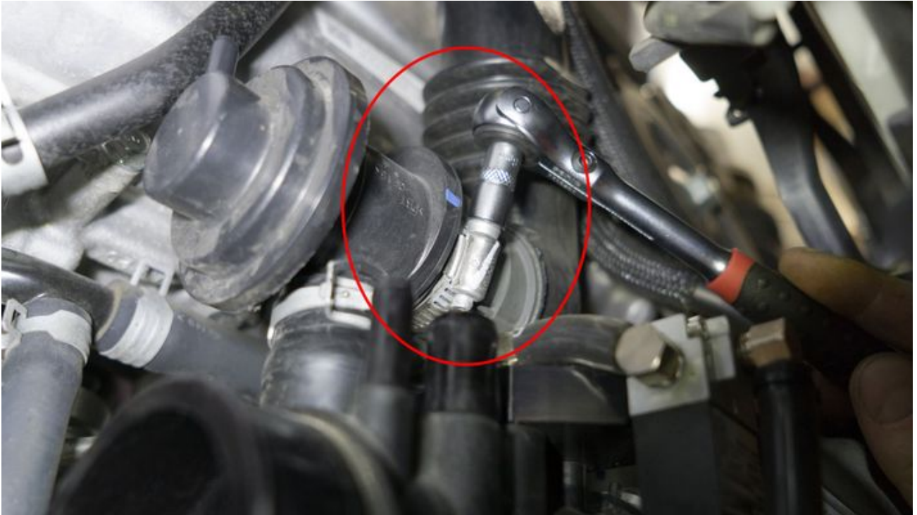
6. Remove (2) 12mm bolts on the factory hot pipe to turbo. You will need a 6" extension for one of the bolts.
