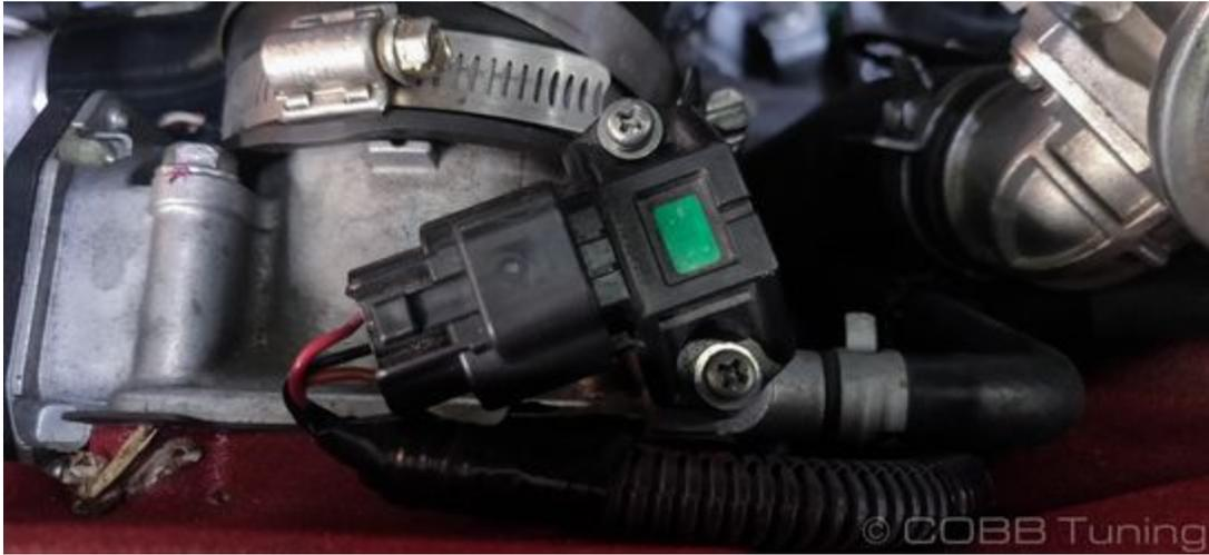
3. Push in the tab and disconnect the map sensor connector from the sensor.
