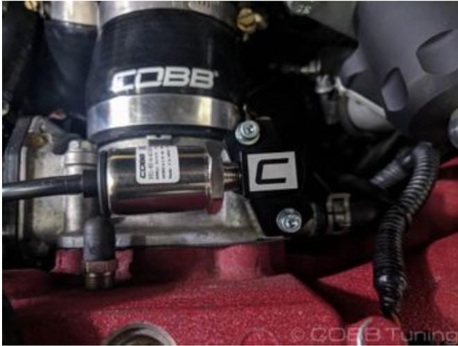
6. With the sensor hand tight, rotate it one and a half more full turns using a 22mm wrench.
