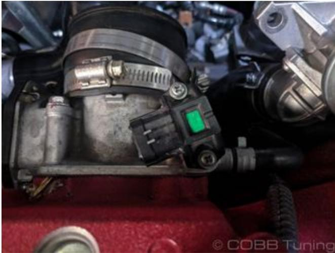
4. Using a screwdriver remove the two screws holding the map sensor to the throttle body. Be careful and go slow to make sure it doesn't strip. If you aren't able to easily remove them, using an impact screwdriver that you hit with a hammer can make removal easier.
