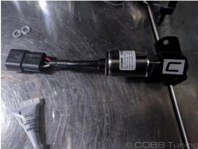
4. Carefully push the adapter into place on the throttlebody. Try to go straight in and avoid crushing or ripping the o-ring.
