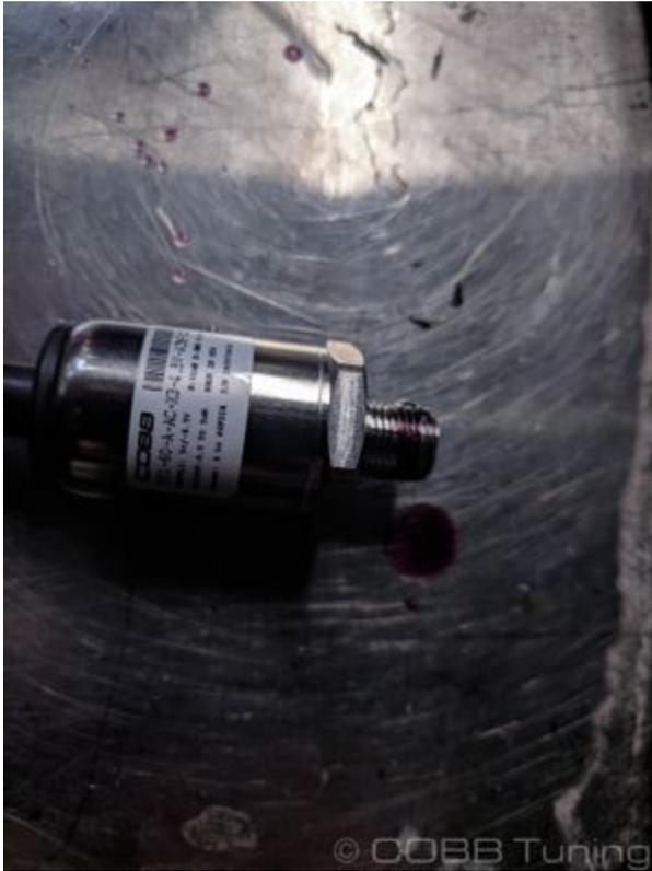
3. Screw the sensor in hand tight onto the adapter.
