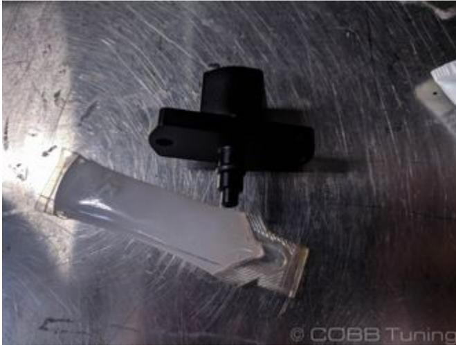
2. Add the included thread sealer onto the threads of the pressure sensor, make sure not to get any on the front portion where it may go into the sensor.
