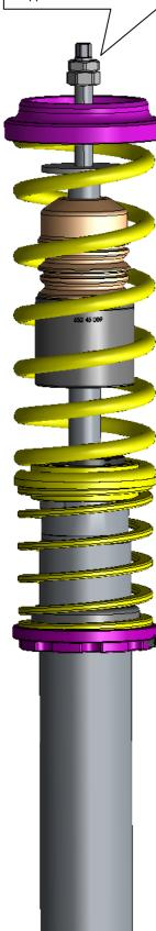
Cut off the dustcover from spring perch on the dashed line. The dust cover is no longer needed.
