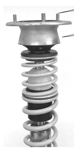
Please install the strut unit to manufacturers recommended settings regarding tightening torque and fixing specifications.
