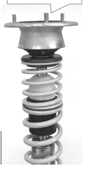
After you have completed installation of the suspension, check the clearance of the wheels/tires to the front suspension system. The minimum clearance at the narrowest point may not be less than 5 mm (0.2 inches). If the wheel/tire does not meet this minimum measurement, wheel spacers may be necessary.
