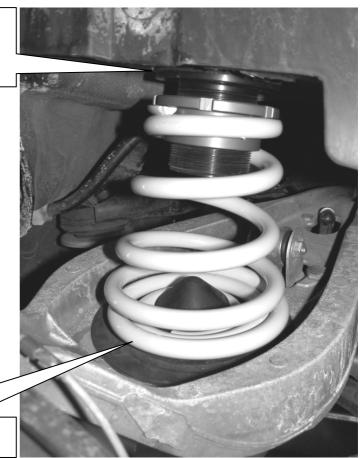
Re-use the original rubber unit at the bottom end of the spring.
