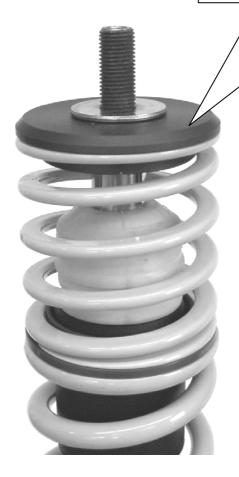
Attach the factory supporting bearing using the supplied stop nut. Tightening torque for the piston rod nut is 50 Nm (37 ft-lb). Use the manufacturers recommended torque settings for installation of the strut and all other fasteners that attach the suspensions to the vehicle.
