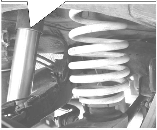
Mount the supplied height adjuster without rubber support between the axle and the lower end of the spring. Tightening torque is 40 Nm (29ft-lb).
