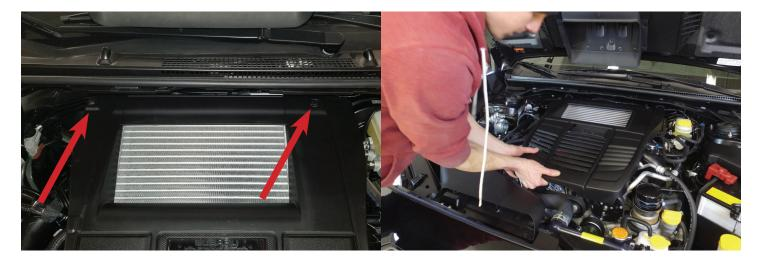
3. Once the engine cover is removed, we need to remove the bracket the OEM cover popped into.
